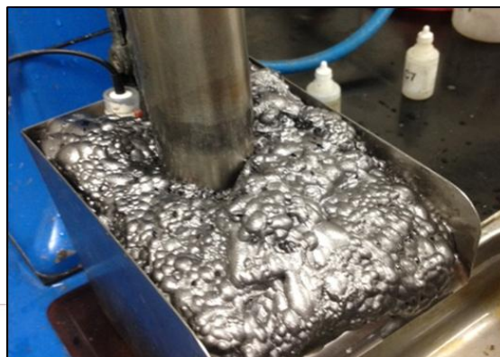
Figure 1 – the simple, chemical free production process of high grade graphite concentrate from the Company’s graphite (GS03 Weathered Composite Rougher Flotation without Collector).
