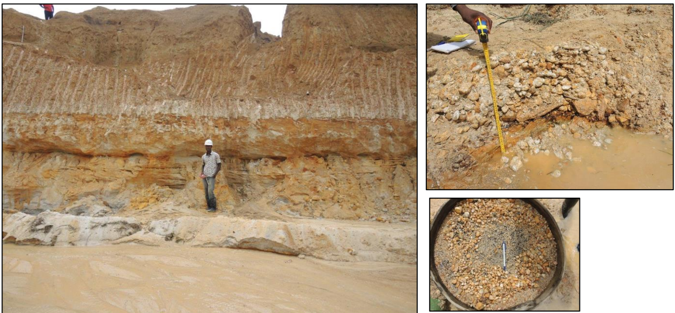
Figure 16. Bulk-sample pit MABS_023 located some 300m south of the Sumbuya Camp. Material from a well-developed basal gravel horizon (top right), with a palaeo-Sewa River stratigraphic signature (note fluvial cross-bedding), was recovered to the Sumbuya plant site for future processing. The heavy mineral assemblage is shown in the wash sieve (bottom right).
