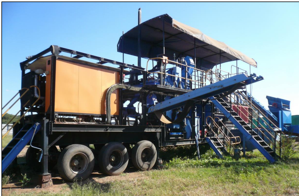
Photograph 2. The 10 tph mobile DMS plant purchased from Dynamic Machinery CC., South Africa.
