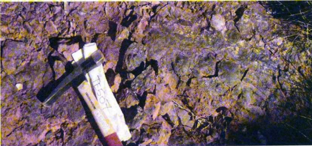
Figure 5b. Outcrop of sample TE507 limonitic breccia with quartz vein fragments close to Magnetic Target 13 (see Figure 3). Note assay data with high Bi (649ppm) and Au (0.33ppm) results.
