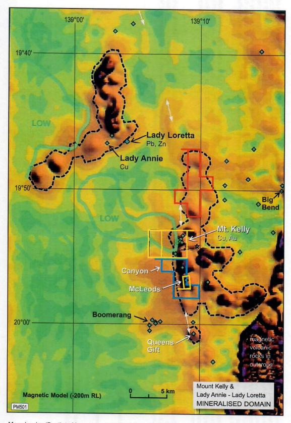
Map showing 'Depth to Magnetic Basement' (='depth to magnetic rock bodies under sedimentary strata') with reference elevation of 200m below sea level, prepared by Kate Nelson, using data from MIM survey on lines at 200m spacing.
