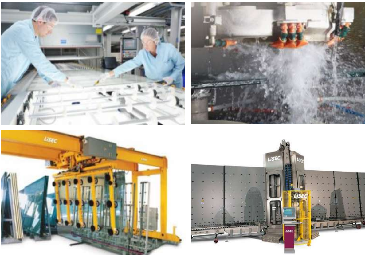
Image 3. (Top Left) Laminated Glass Processing Line, (Top Right) Glass CNC Cutting Line, (Bottom Left) Automatic Crane Stocking System, (Bottom Right) Automatic Glass Edging
