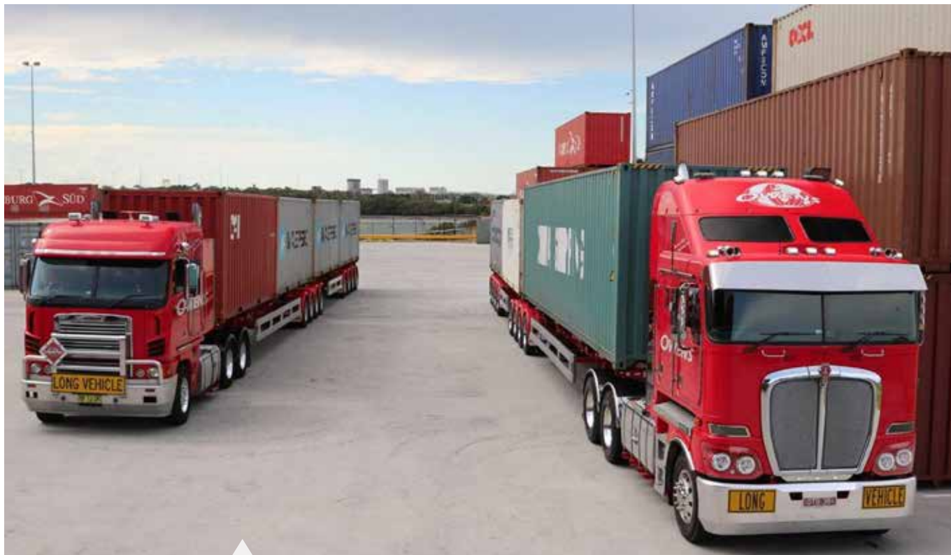
New super B in Brisbane carting from the depot to the wharf. It gives us the capability of moving 4 20ft containers per truck per trip.
