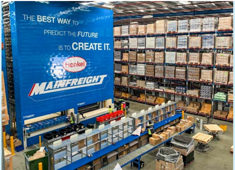
The big blue shiny machine is the VLM and the tote locations opposite to that is the Put Wall
