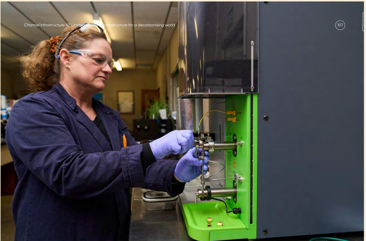
Laboratory technician at Independent Petroleum Laboratory setting up specialist equipment for fuels quality testing
