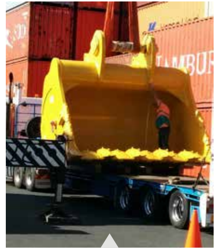
Loading an oversized bucket to road to a mine site in NSW
