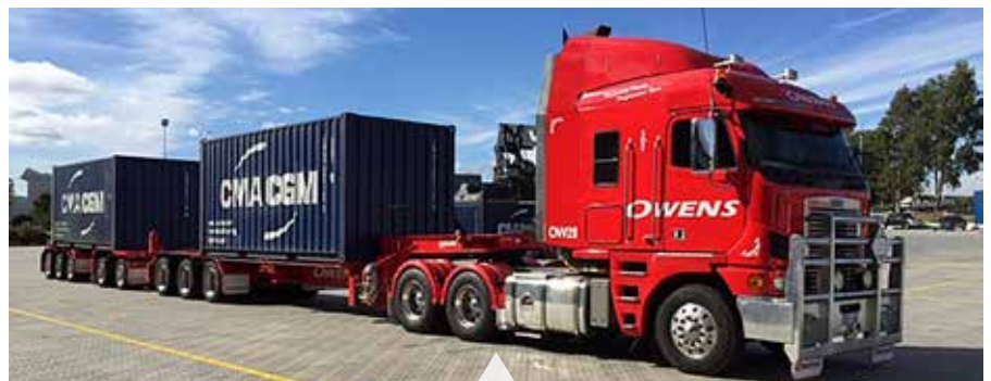
This unit is currently doing two runs a day out to the southwest of WA, which is just a short haul of 400km per round trip. The product we are loading is waste engine oil heading back to Singapore to be refined. Each container is loaded with a flexi bag with holds 26000 litres of bulk oil and weighing in at over 26 tonne per container.
