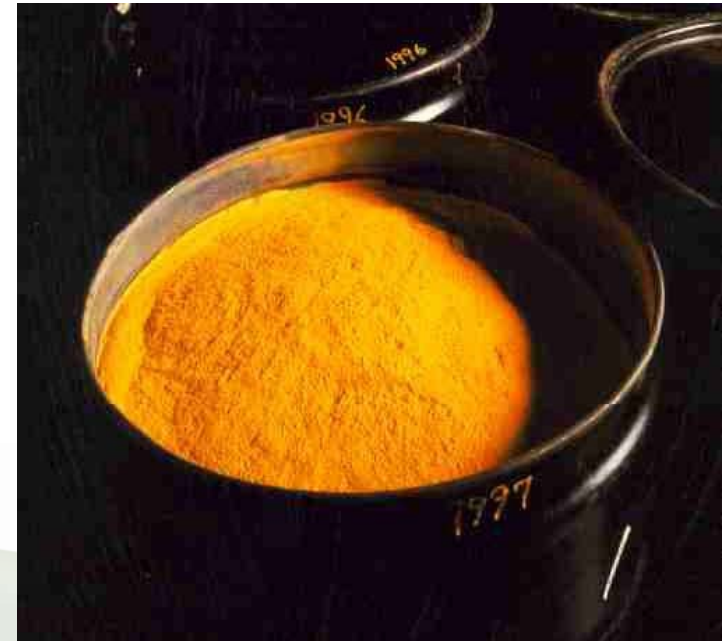
Yellowcake – typically the first stage product recovered when processing uranium ore.
