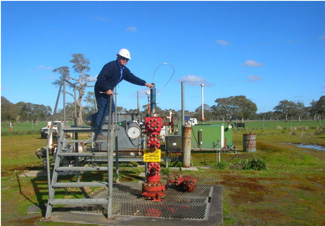
Figure 1: Adelaide Energy's Field Superintendent, Russel Campbell at Haselgrove 1 Production Tree showing the surfactant injection line
