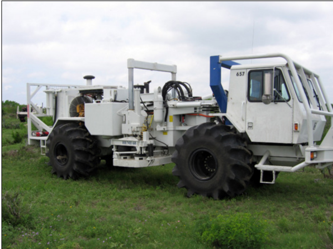
Vibroseis truck acquiring seismic data over Yellow Rose - June 2007
