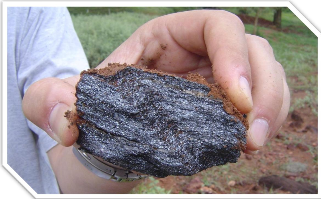
Figure 5 - Example of high grade mineralisation (up to 66% Fe) contained in the hydrothermally enriched portions of Passabem that will be targeted through ground magnetics and drilling.
