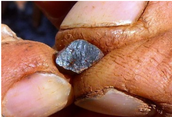
Figure 12 - concentrated haematite iron fragment in pisolite from Spearhole Channel Iron Deposit
