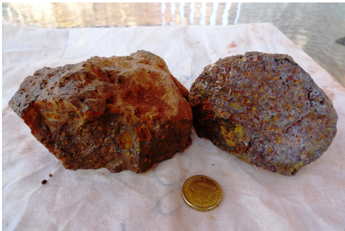
Plate 5 - example of fragments of Channel Iron sub-crop, showing well formed pisolites and petrified wood fragments
