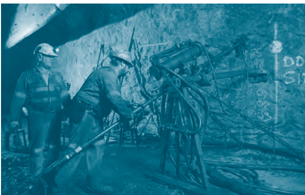
Underground Diamond Drilling
