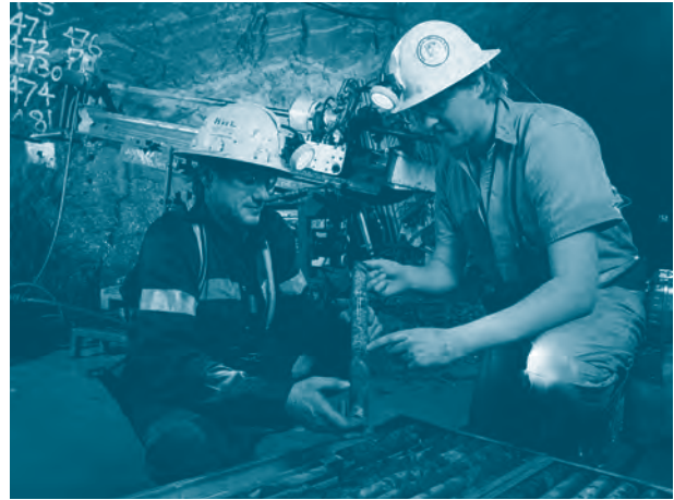
Underground Diamond Core Sample
