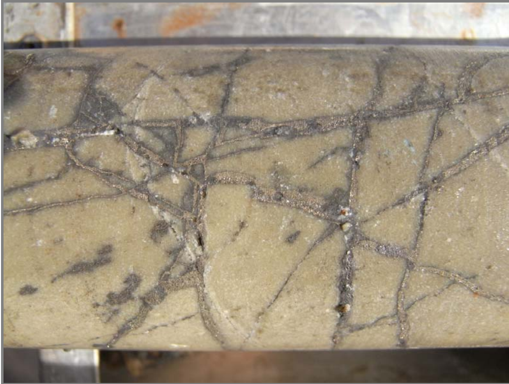
Figure 2: Typical stockworking sulphide veins from drillhole Round Hill North B (at 54m depth).
