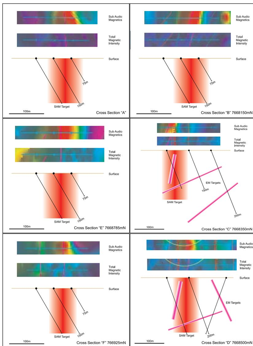
Figure 5: Drill Traverses A-F diagrammatically represented in Cross Section with SAM and TMI plan view slices.
