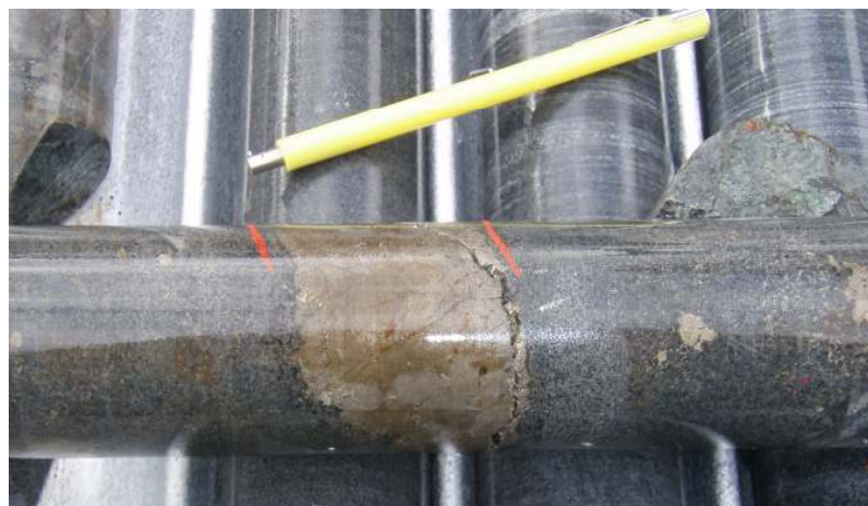
MTDD008 6cm wide massive sulphide stringer (pyrrhotite and pentlandite) near lower contact in Proterozoic dyke (NQ Core), 759m depth.
