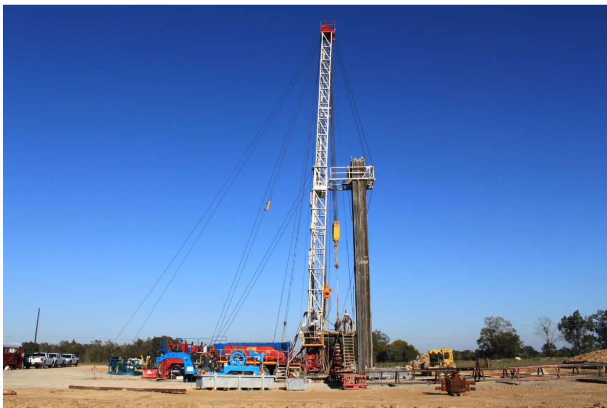
Crews on the HM Brian No.1 well pulling the drill string out of the hole prior to logging
