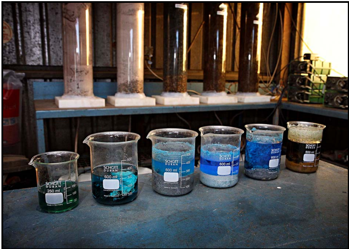
Figure 1. Samples of copper and nickel in solution, from column testing.
