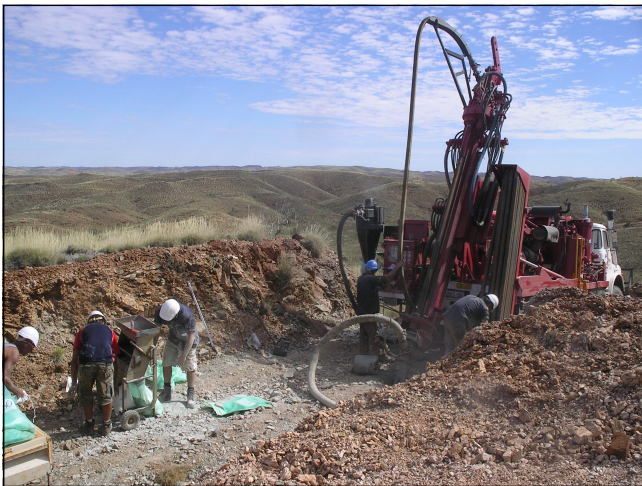
RC drilling in exploration trench at Big Hill - July 2008
