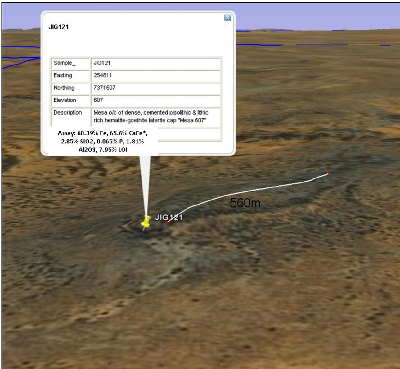
**Figure 2:** JIG 121 rock chip sample at Mesa 607; Jigalong Project
