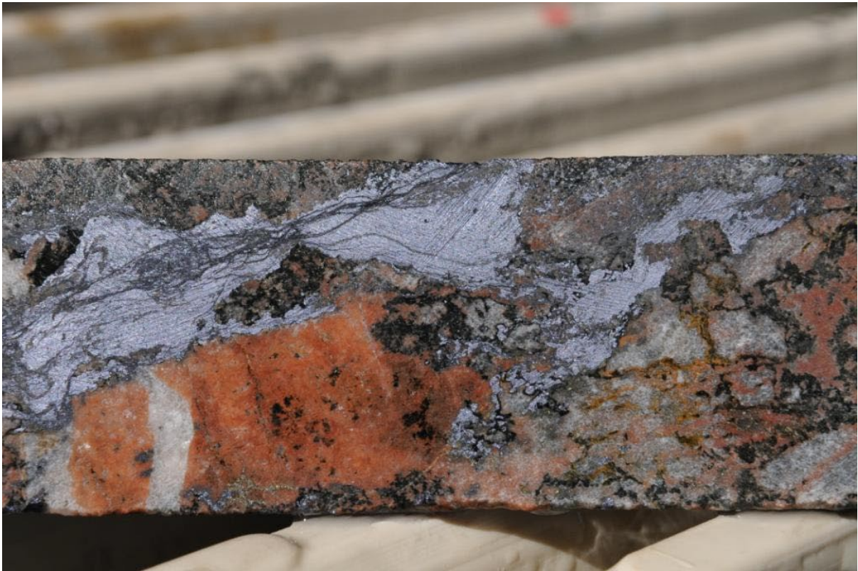
Figure 14: High-grade Molybdenite as Massive Veins and Stylolites in Lanham's Shaft Drill hole LAD0003
