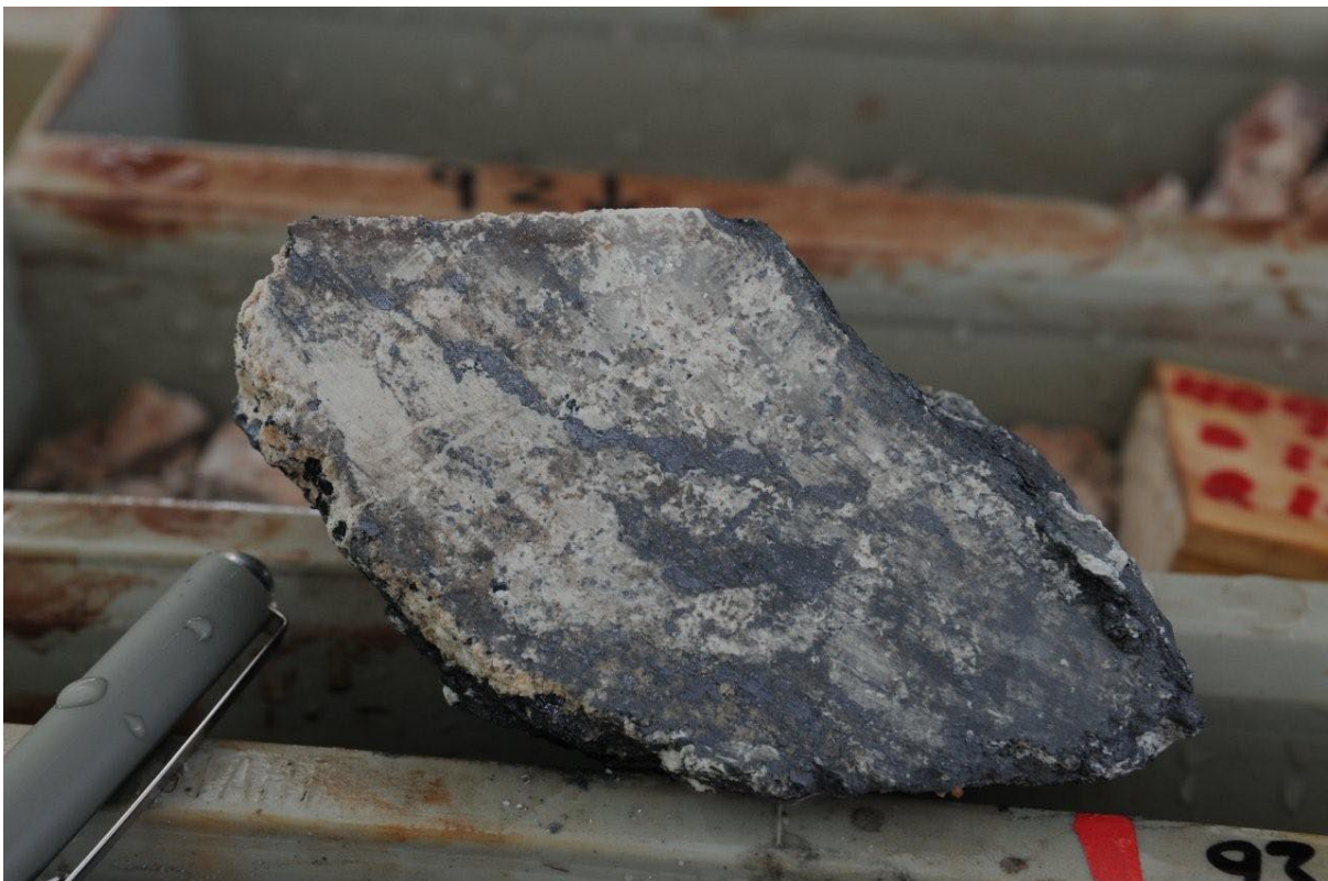
Figure 7: Little Wizard Molybdenum/Rhenium Bonanza mineralisation in Drill hole MDQ0279
