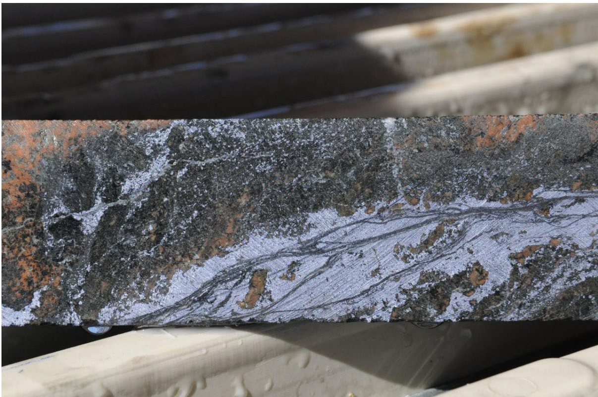
Figure 13: High-grade Molybdenite as Massive Veins and Stylolites in Lanham's Shaft Drill hole LAD0003
