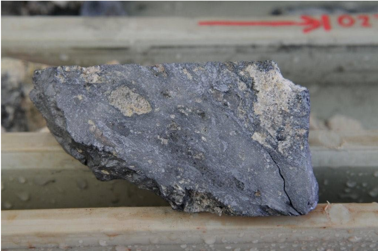
Figure 8: Little Wizard Molybdenum/Rhenium Bonanza mineralisation in Drill hole MDQ0279
