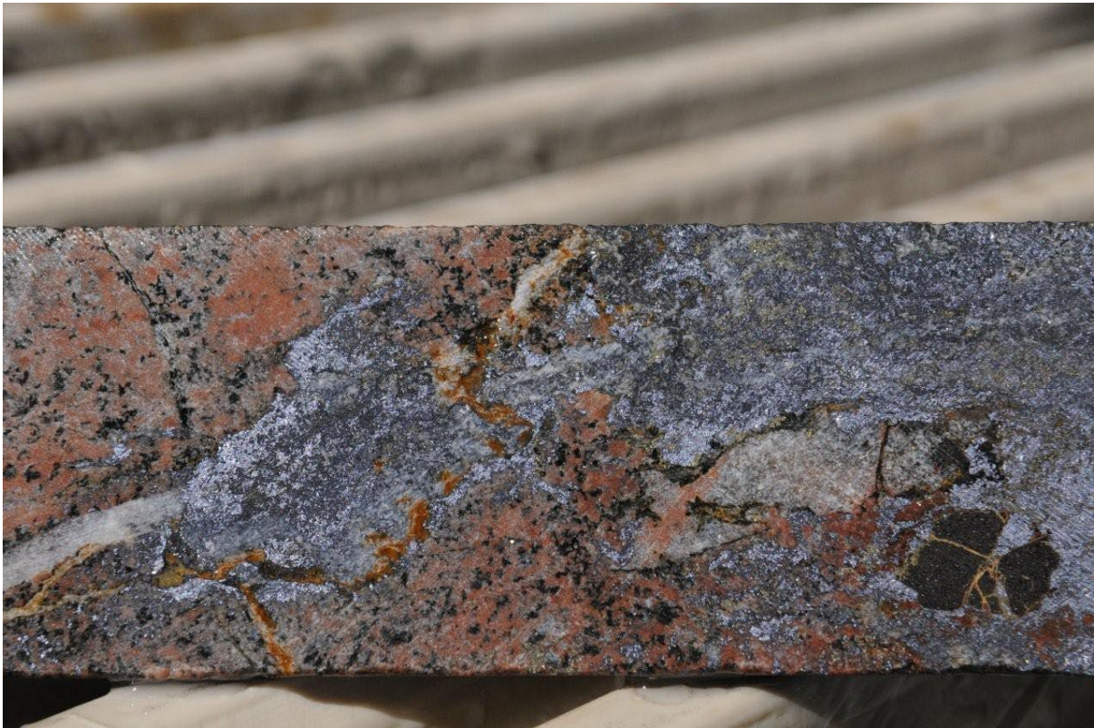
Figure12: High-grade Molybdenite in Brecciated Calc-Silicate with Uranium minerals (Uranite and Coffinite) in Lanham's Shaft Drill hole LAD0003
