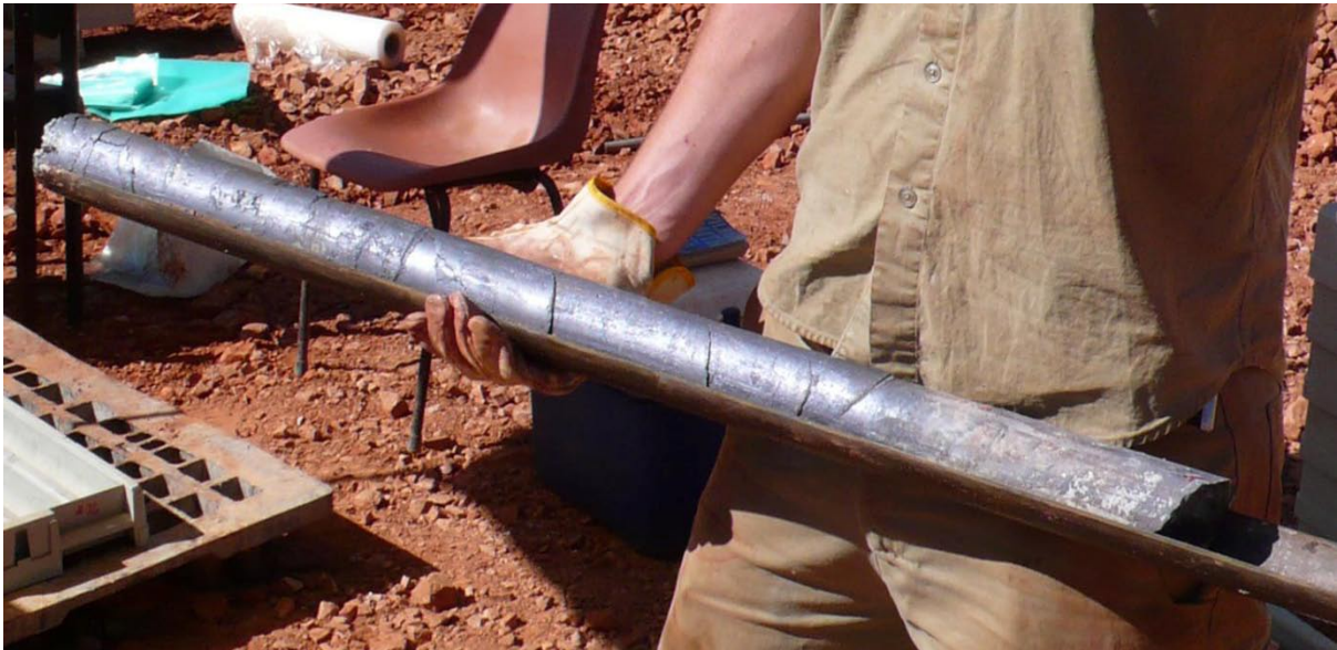
Figure 4: Little Wizard Molybdenum/Rhenium Bonanza Discovery hole MDQ0264 showing High-grade Massive Molybdenite mineralisation
