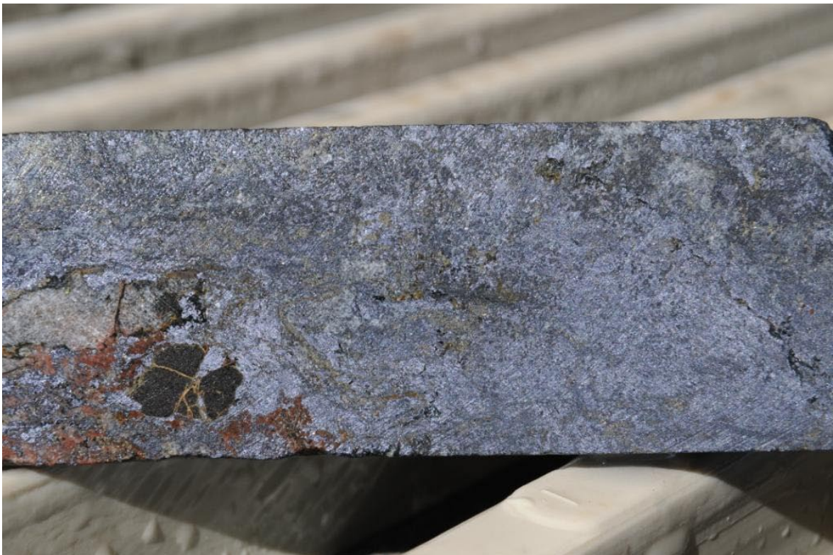
Figure 15: Massive Molybdenite with Uranite and Coffinite in Lanham's Shaft Drill hole LAD0003
