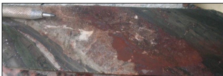
Figure 2: Dolomite vein with earthy haematite and associated chalcopyrite (AS09D03: 720.0 m)
