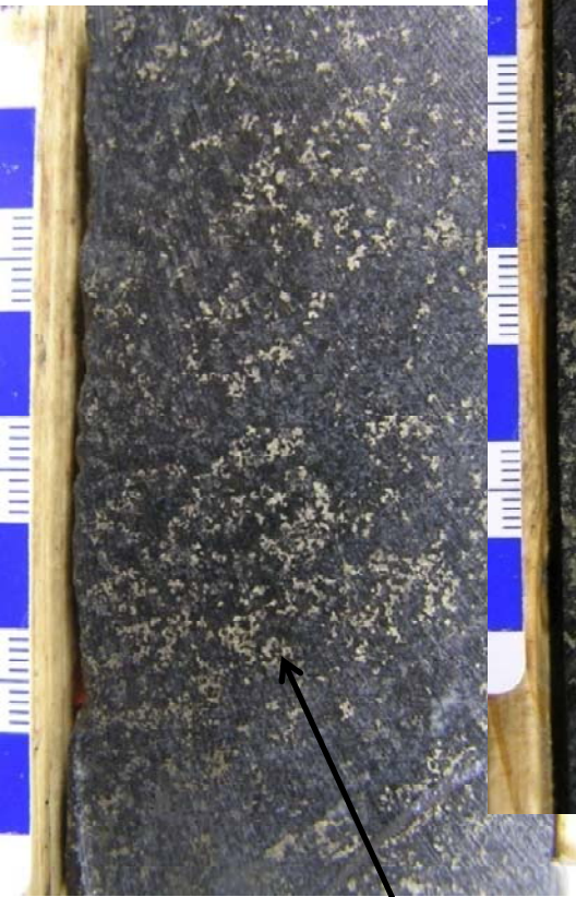
Disseminated Sulphide (~3-5g/t PGM, ~0.4% Cu & ~0.3% Ni)
