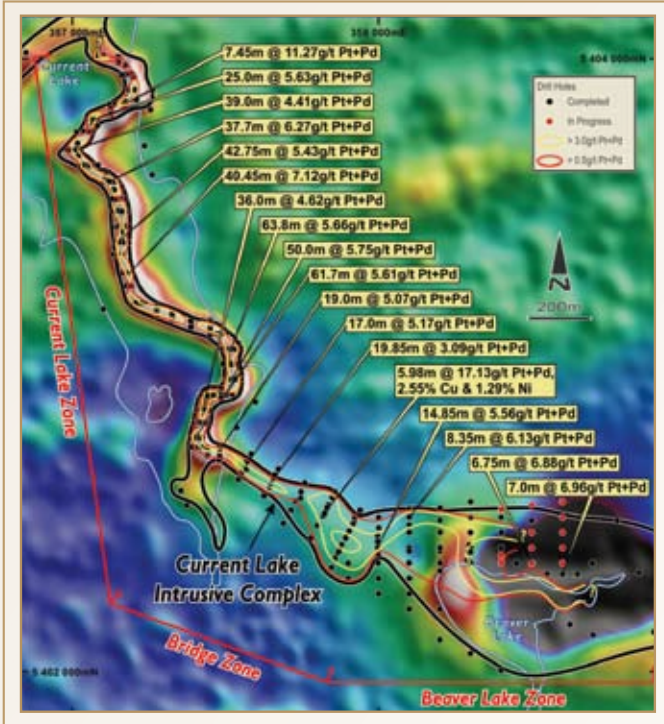
Figure 3. Drilling in the Current Lake – Beaver Lake Area
