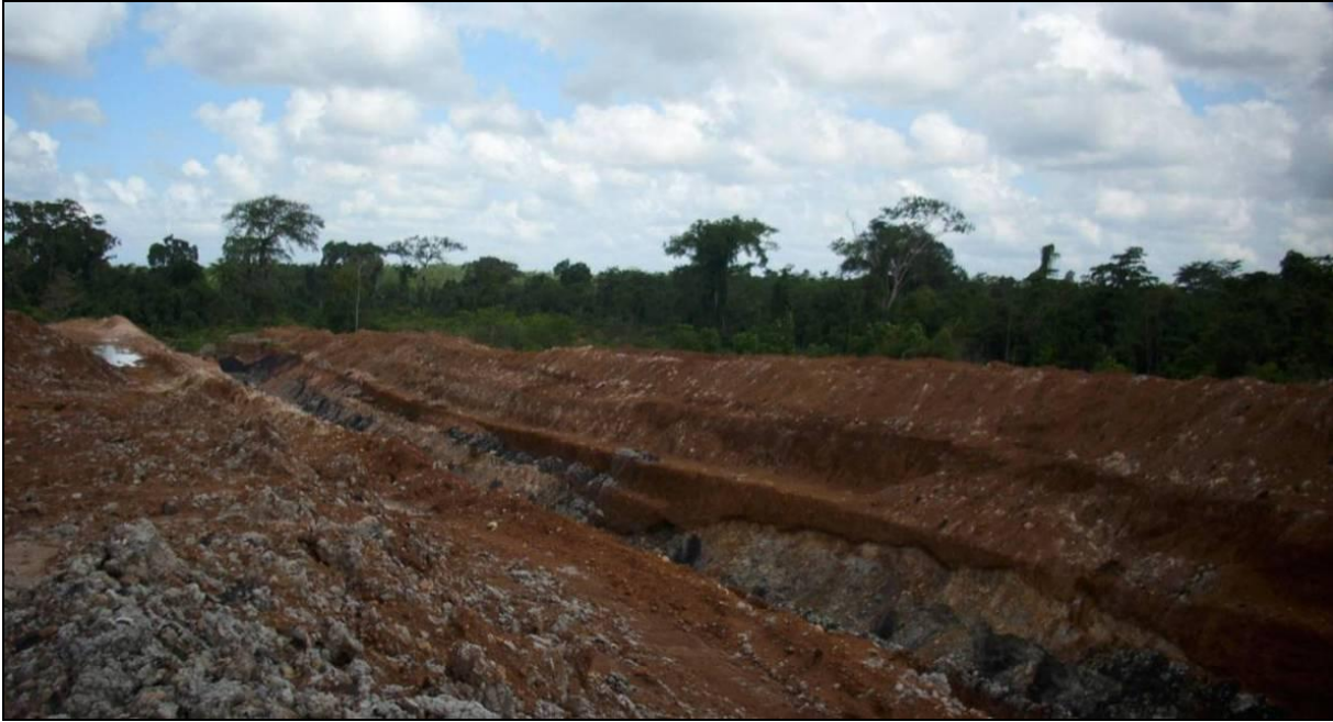
Figure 6.2. Strike view of DP pit with in-situ coal seams exposed in highwall.
