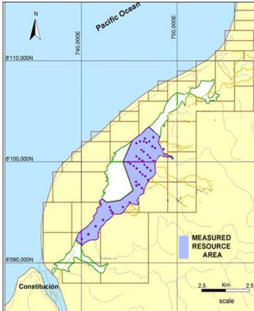
Figure 1. Plano Prospect, outlined in green, showing the locations of 41 auger drill sites, and the area where a measured resource has been calculated. Indicated and inferred resources have been estimated for the remaining areas of Plano Prospect, as shown in Figure 2. Modern dunes cover the concession area west of Plano, and Katy Prospect is located to the east.
