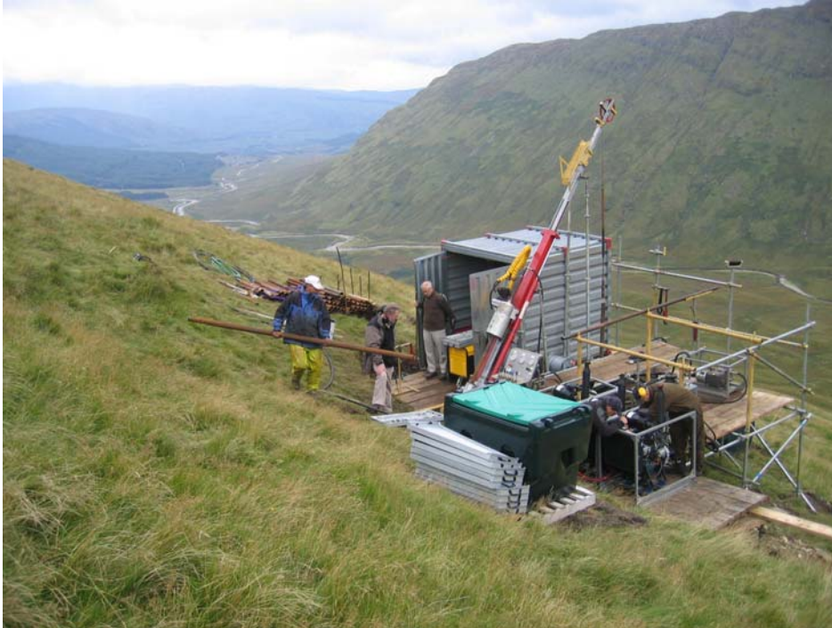
Photo 1: Drilling at Cononish using Scotgold's Explorer Plus MD3 diamond drill rig
