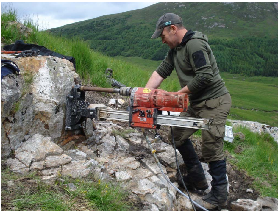
Photo 2: Drilling at Bienn Udlaidh using an electrically-operated, hand held rig developed by Scotgold and Priority Drilling
