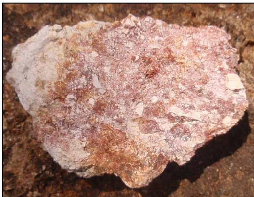
Photo C: Clay and silica altered brecciated host interpreted as a deformed mafic intrusive Specimen is about 10cm across.
