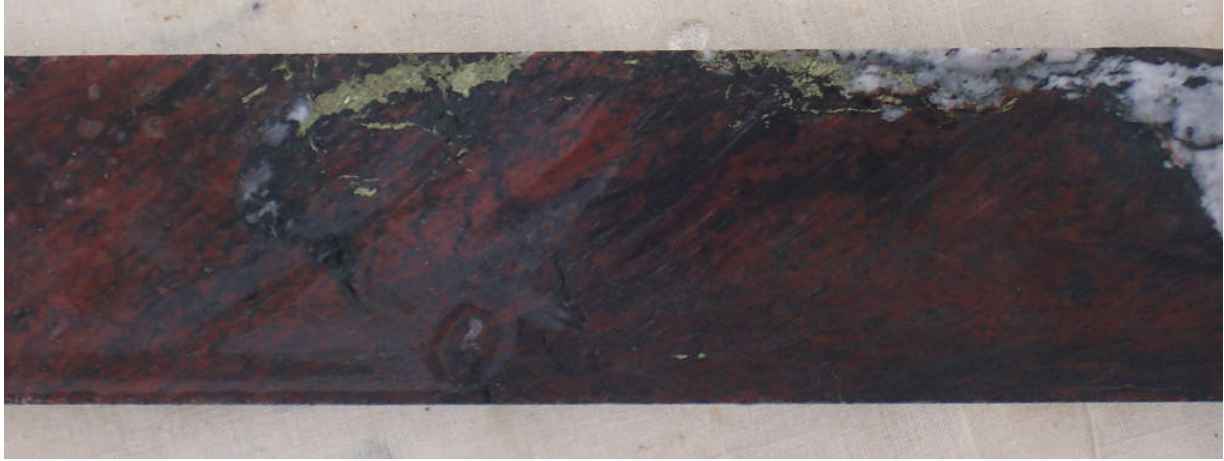
Figure 1 – chalcopyrite-magnetite-chlorite vein in haematite altered porphyry
