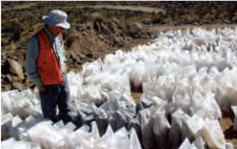
Figure 3.5.1_1 Los Pumas Manganese Project RC Bulk Reject Bag Farm
