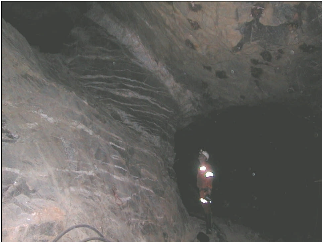
Example of flat lying quartz splays off the steeply dipping main reef. Photo taken during mining at Golden Crown
