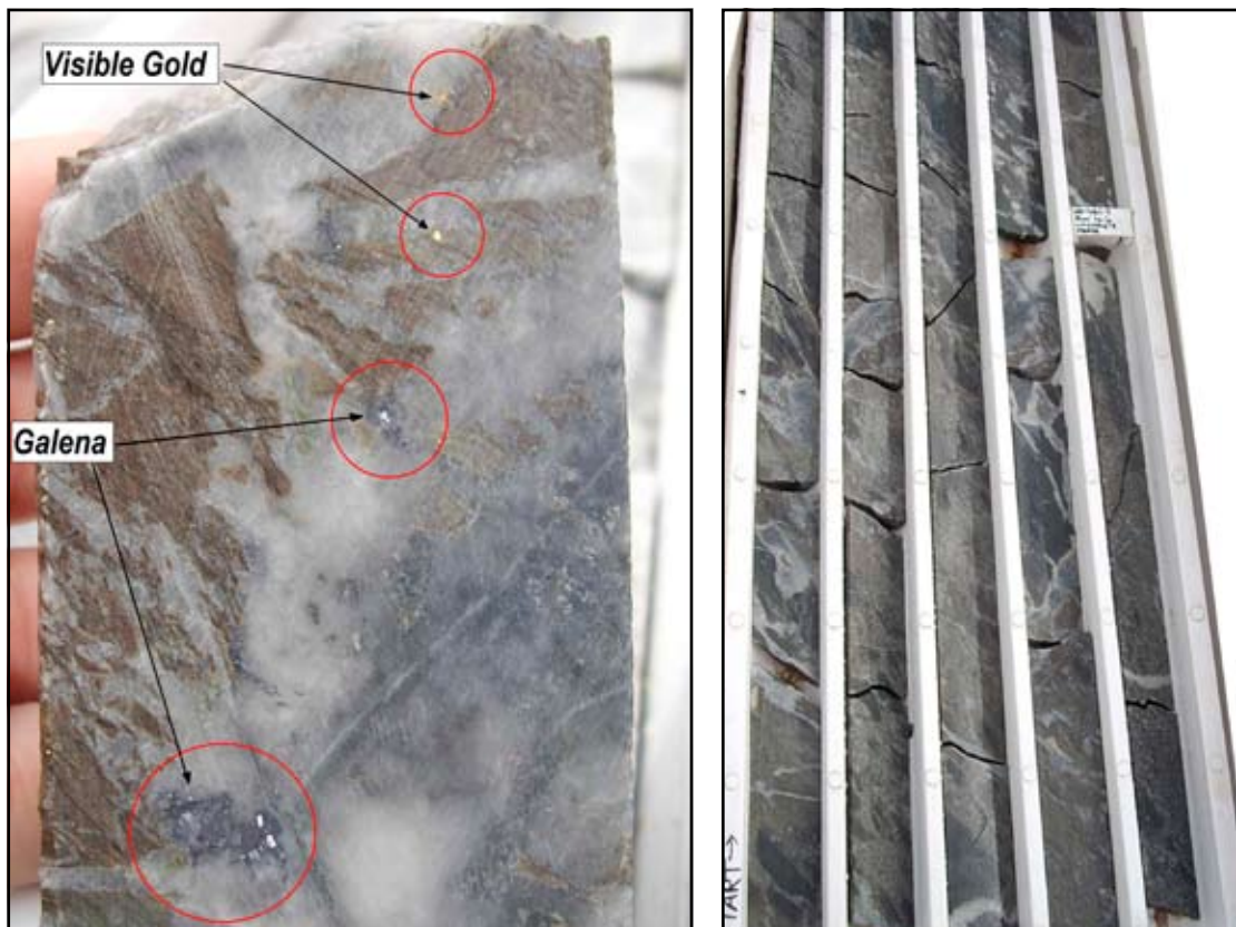
Figure 12. Diamond drill-hole CMC0003 at Black Swan South showing visible gold in quartz that returned 6.1 metres @ 7.2g/t Au from 458 metres.
