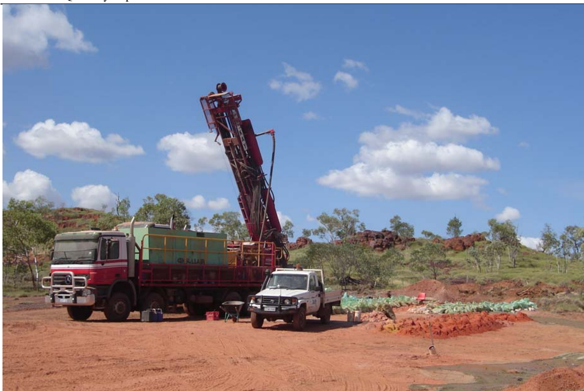
Figure 4. RC drilling at the Sandiego Prospect. The Sandiego gossan is on the skyline.
