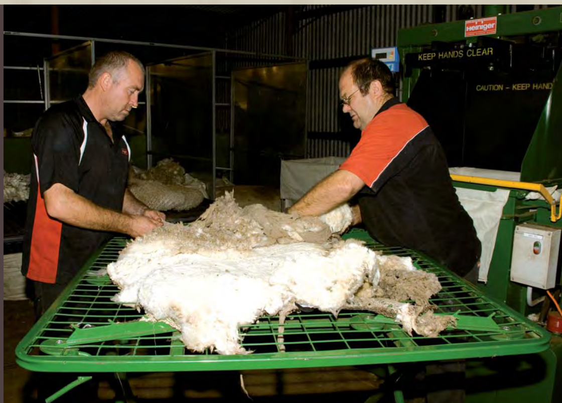
Newly developed net stretcher for removing the fleece
