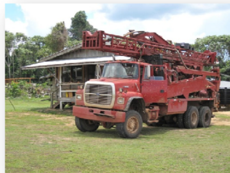
Images of the truck mounted Drilltech D-12 truck mounted rig and support equipment, at the Hicks base camp West Omai Project, Guyana.
