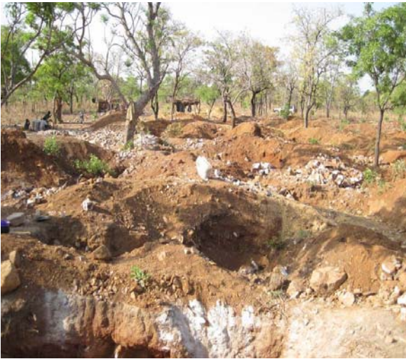
Artisanal workings exploiting north-south laminated quartz vein at Julie
