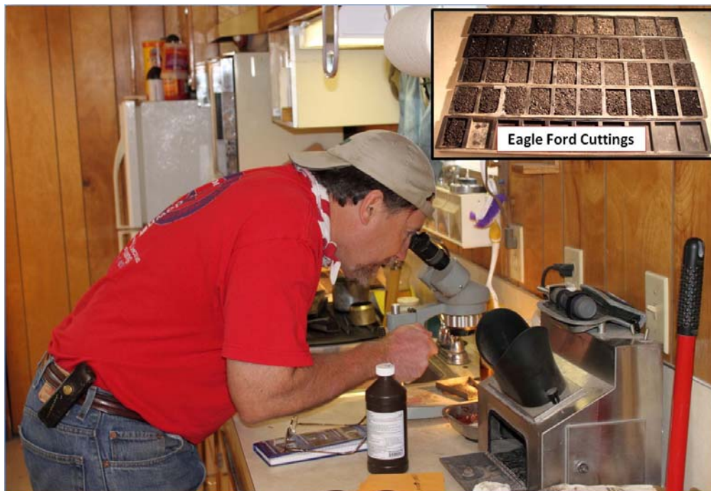
Antares' Chief Scientist, Greg Shoemaker, analysing Eagle Ford shale samples under a microscope. The Eagle Ford shale was encountered at 10,870 ft with excellent hydrocarbon shows.
