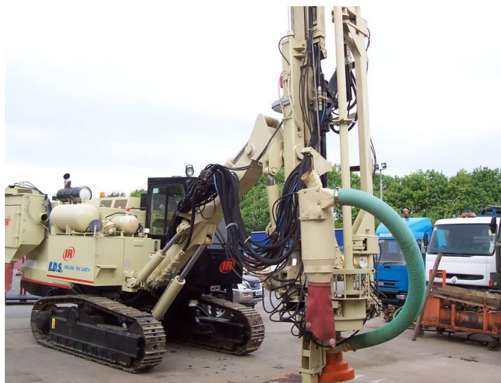
Figure 4 – EDS RAB Drill Rig
