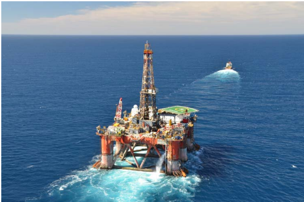
11 Dec 2010 - Semi submersible rig "Ocean Patriot" under tow to New Seaclem 1, PEP 11.
