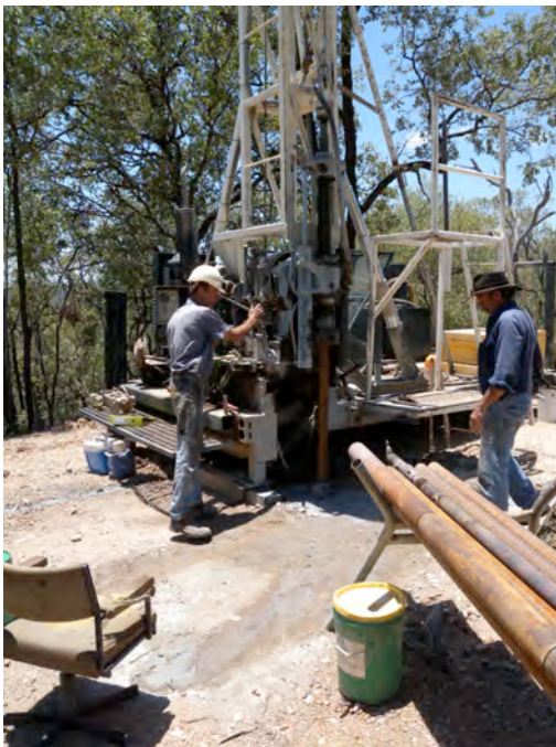
Core drilling on EL 3325
