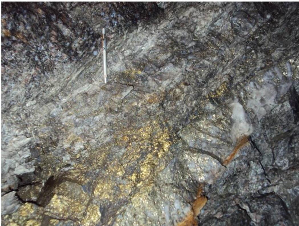
Figure 6: 67 cm wide quartz-sulphide vein which assayed 79g/t gold (Shaft 1, Sample 130009, -24 Level)
