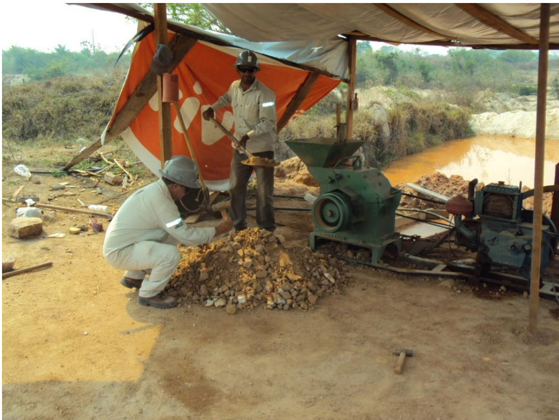
Figure 4: Processing of a bulk sample at Cidinha Prospect, Alta Floresta Gold Project. Note the typical garimpeiro pit, now filled with water, in the background.
