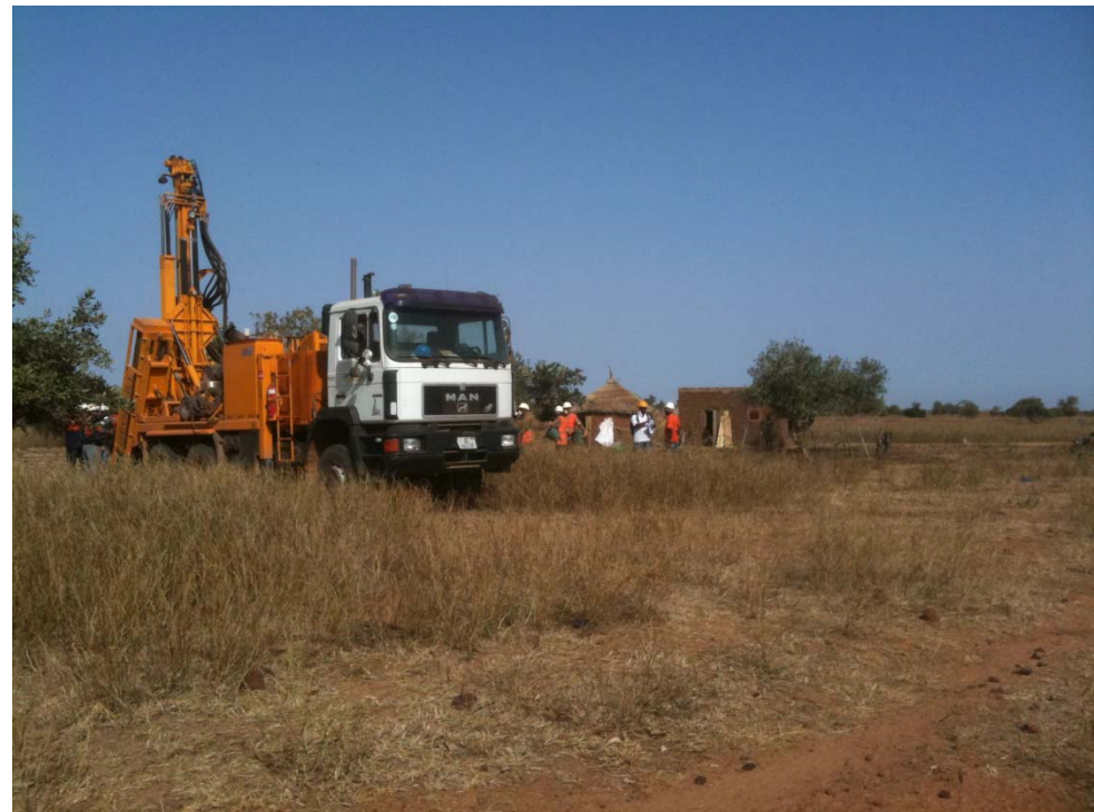
Aircore rig drilling on the Madougou Permit
