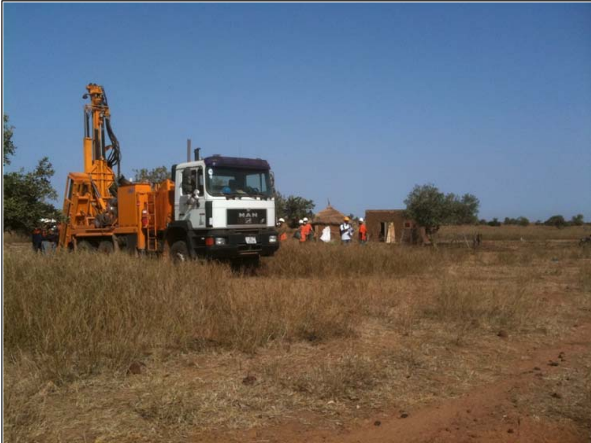
Figure 2: Aircore rig working on geochemistry drilling on the Madougou Permit November 2010.
