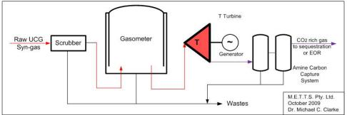
Figure 5b. UCG post power generation carbon capture
