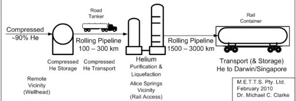
Figure 3. An Extended Helium Rolling Pipeline
