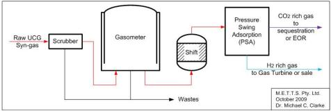
Figure 5a. UCG hydrogen production and power generation
