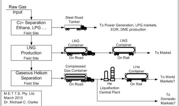
A three product production and logistics schematic emphasising the use of the rolling pipeline
