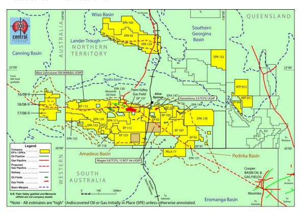
Ooraminna 2 is the first conventional well in Central's Phase Two Amadeus Basin drilling programme and will target up to 2 trillion cubic feet of gas (TCFG -"high" estimate) in a fractured reservoir that flowed gas to surface in 1963 but was not effectively tested. Directional drilling techniques will be used on Ooraminna 2 to increase the number of anticipated vertical fracture systems with potential to host gas. This technique will be used to maximise the well's productive capacity.
