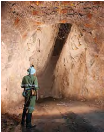
Narrow vein stoping underground
