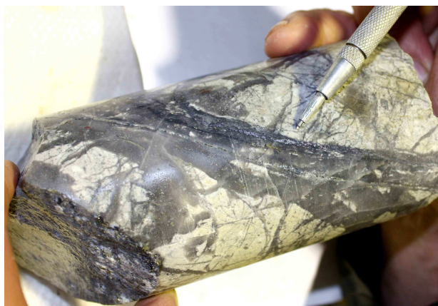
Photo 1. DUNDD004. Mo mineralisation ( Up to 0.44% Mo ) from high grade quartz stockwork style veining within silica – sericite altered rhyolitic porphyry.
